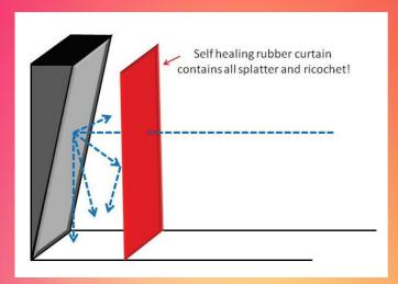
It is mainly used for hanging curtains that protect covering steel trap and concrete backs for deflection. Shooting range rubber sheets has outstanding strength, resilience, and resistance to cutting and tearing
